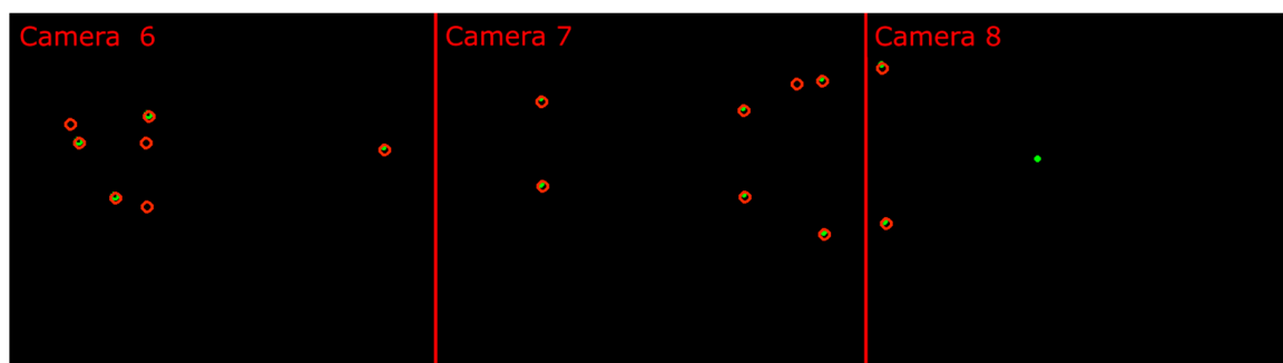
Figure 6. Images of three cameras used for pose initialization. Green dots are markers detected by the cameras, while the red circles are projected points based on the pose and the known 3D marker coordinates.
