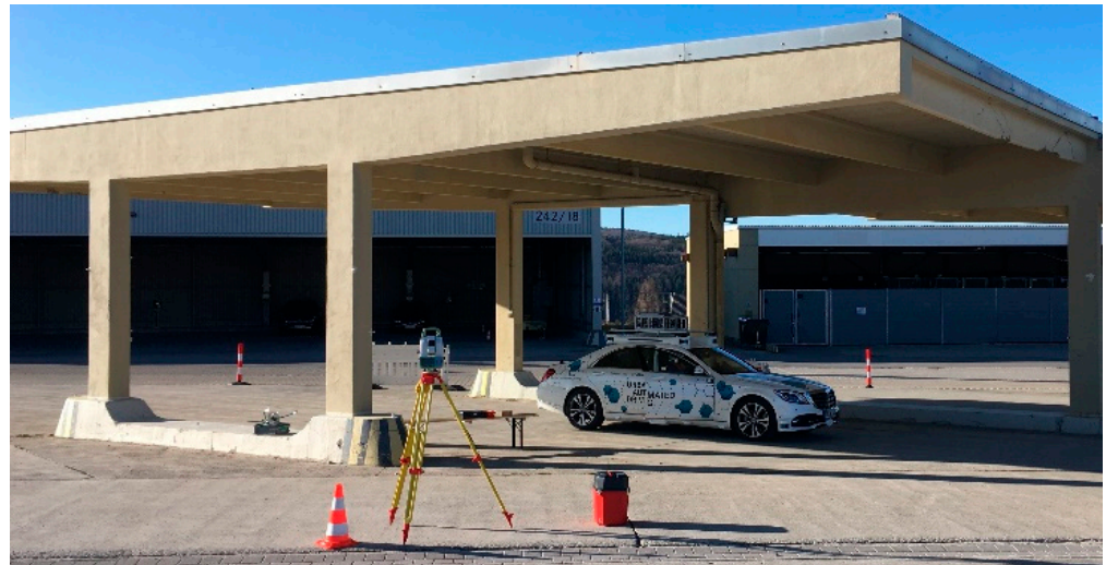
Figure 2. Setup of the tracking system at the test site, consisting of one MS60 (on a tripod in the front) and a camera rig on the roof of the car.
