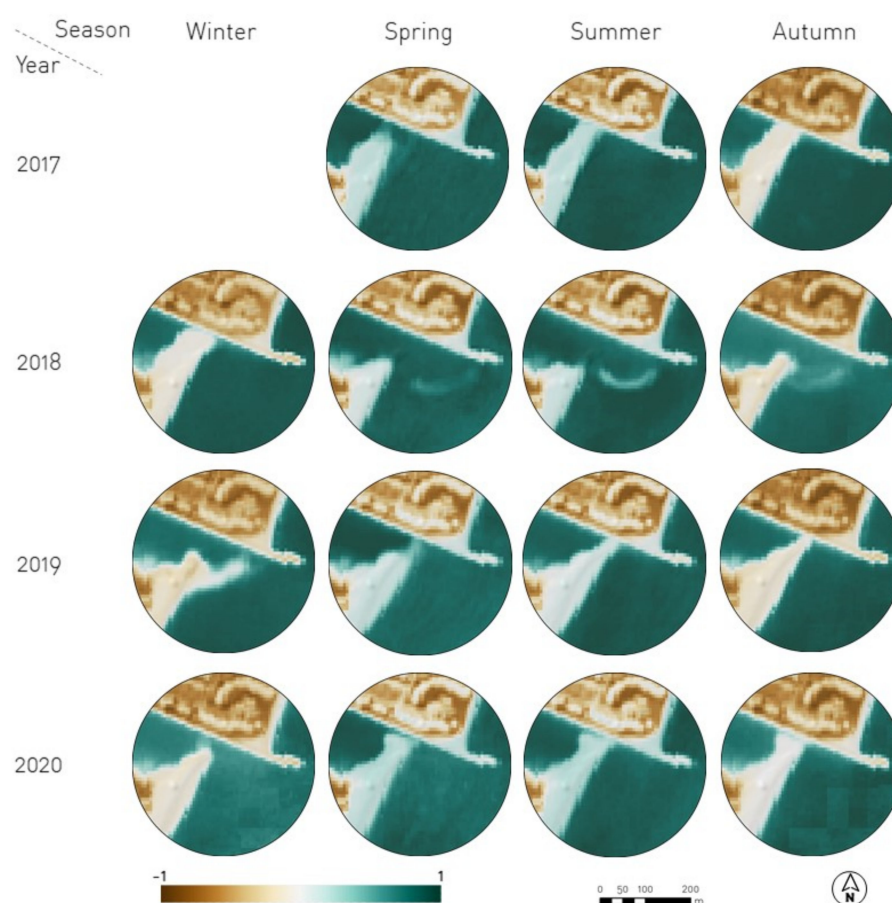
Figure 8. Seasonal climatologies using Sentinel-2 L2A images and NDWI index for the Guadiaro river mouth and its dynamic sand bar between spring 2017 and autumn 2020. Scale 1:3500.
