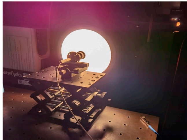
Figure 24. Placement of the telescope and integrating sphere light source during radiation response test.
