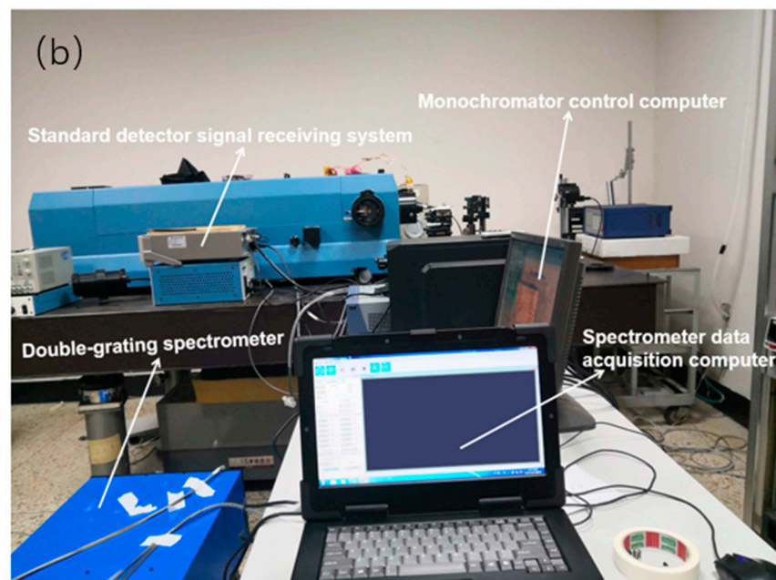
Figure 16. Water vapor absorption band (758–880 nm) spectrum calibration system: (a) Water vapor absorption band (758–880 nm) spectrum calibration flow chart; (b) The instrument of the water vapor absorption band (758–880 nm) spectrum calibration system and the working principle.
