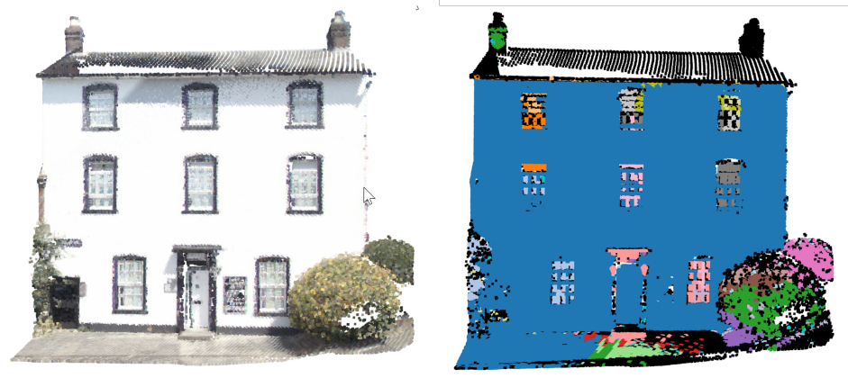
Figure 12. Example of building segmentation. Raw point cloud collected from terrestrial laser scanner with RGB values. Source OS © Crown copyright and database rights 2022.
