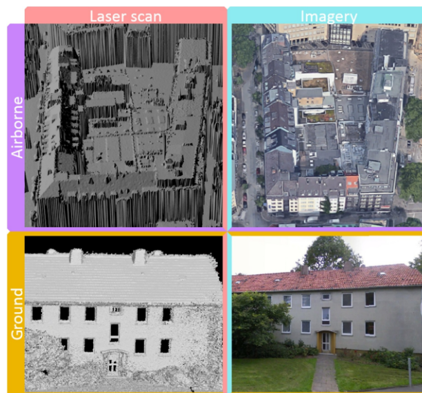
Figure 5. Data commonly used for 3D building reconstruction. Reprinted with permission from Ref. [50].
