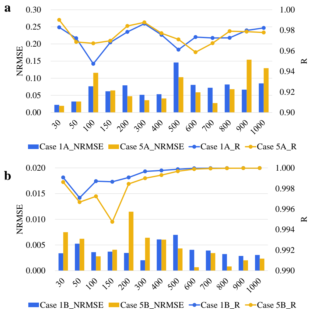
Figure 12. The inversion accuracy of (a) ST and (b) SS for monthly and daily data at different depths using the ConvLSTM model.
