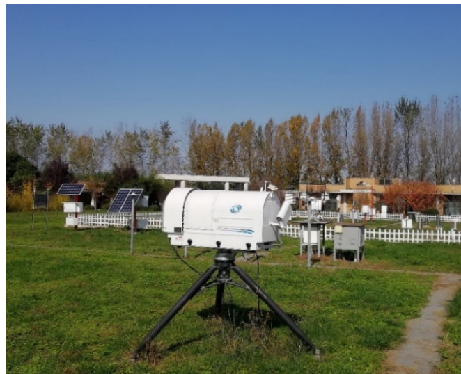
Figure 2. The multichannel microwave radiometer used for this experiment.
