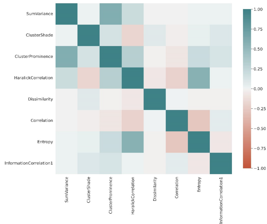
Figure 5. Correlation matrix plot of the 8 least-correlated textural features generated from the panchromatic image.
