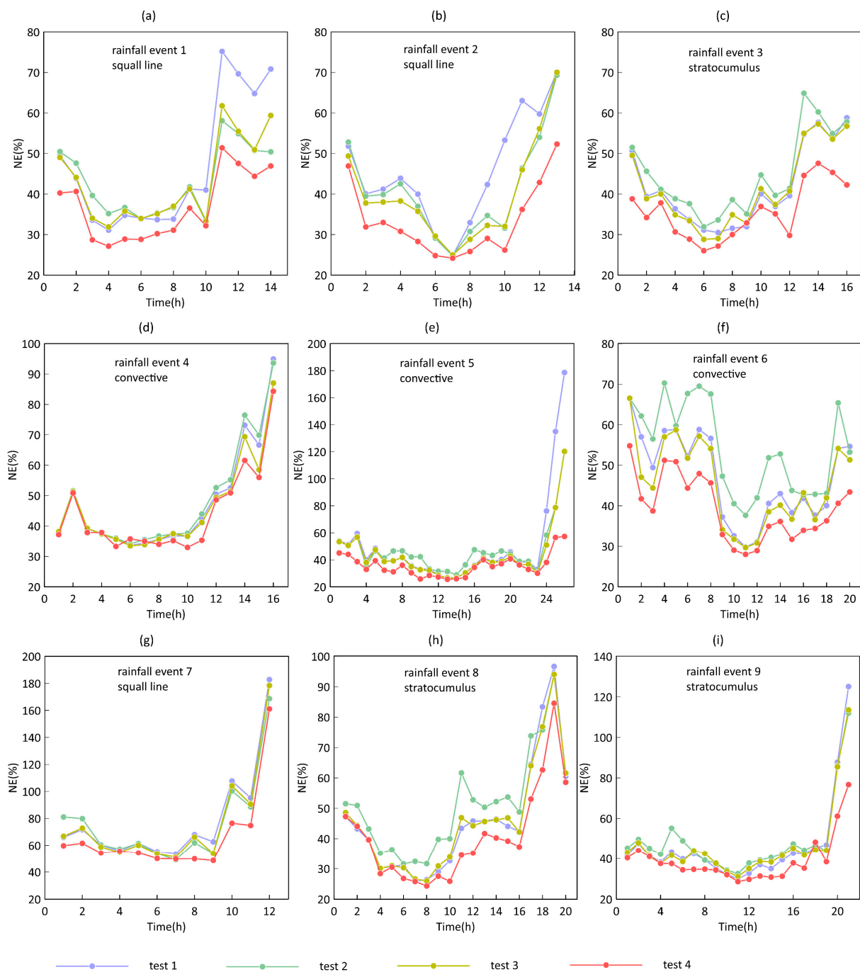
Figure 5. (a–i) Time series of NE values for the rainfall event 1–9. The QPE performance at CRQI > 0.9 was evaluated. The purple, green, yellow, and red lines represent NE values in tests 1, 2, 3, and 4, respectively.
