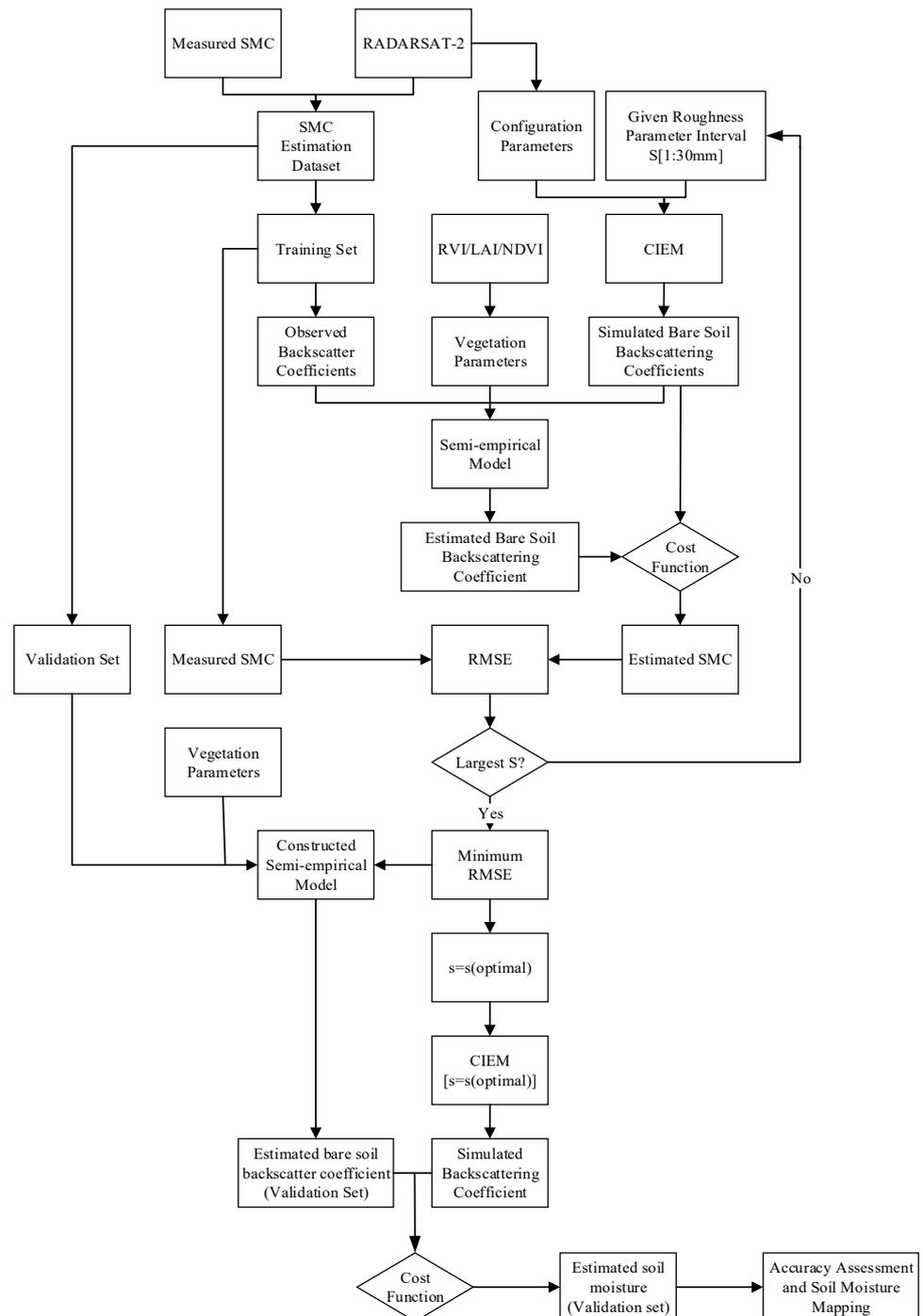
**Figure 3.** Workflow of soil moisture retrieval.
