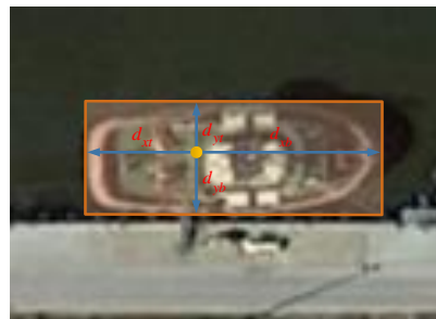
Figure 4. The offset of the anchor-free detection branch. The distances from the current location to the left, right, top, and bottom side of the bounding box are represented by d_{xt} , d_{xb} , d_{yt} , and d_{yb} , respectively.
