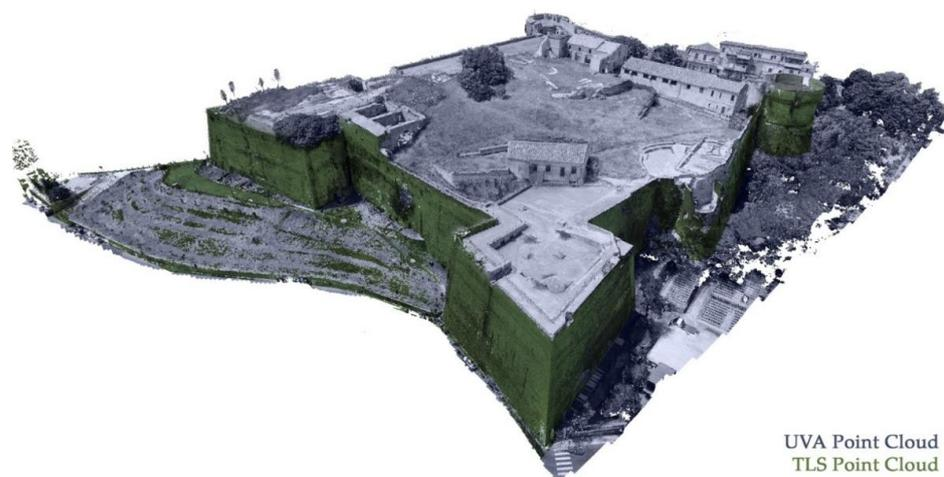
Figure 6. Integrated TLS (green) and UAV (violet) point clouds.
