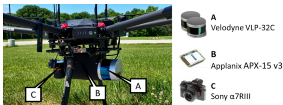
Figure 1. The UAV-1 mobile mapping system and onboard sensors used in this study.
