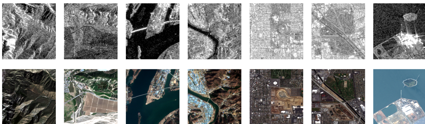
Figure 6. The examples of the SEN1-2 dataset. The first row is SEN-1 data, representing SAR images, and the second row is SEN-2 data, representing optical RGB images. Best viewed in color.
