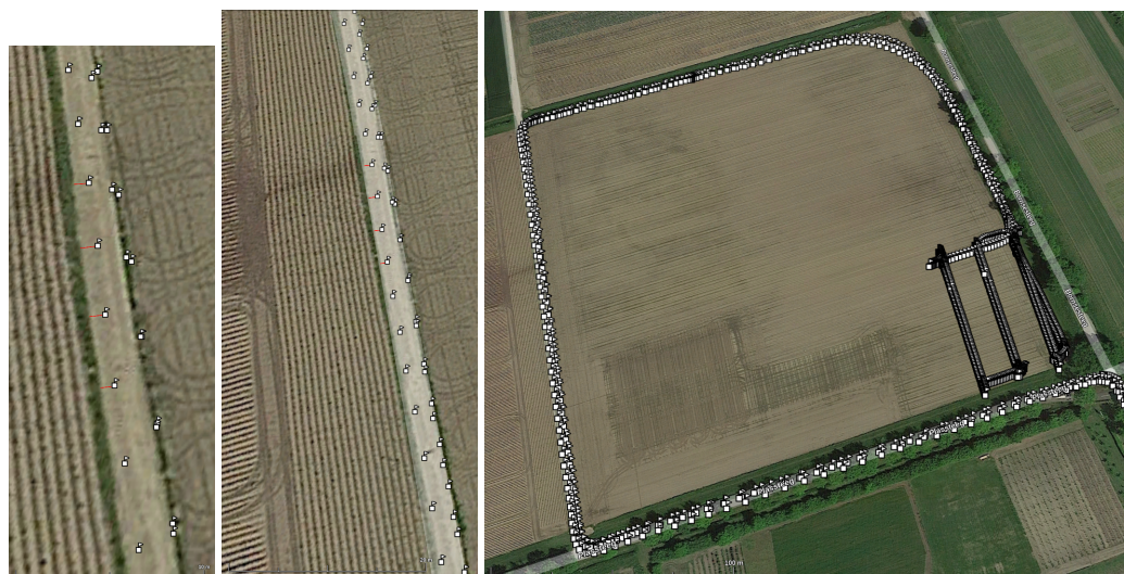
Figure 12. Detail of TPSD WARTK trajectory, showing (with a zoom from the right to the left ) the consistency of the tractor distance to the path border (representative red segments at the left-hand plot with lengths of 97 cm, 96 cm, 91 cm and 83 cm) with the expected WARTK accuracy at decimeter level.
