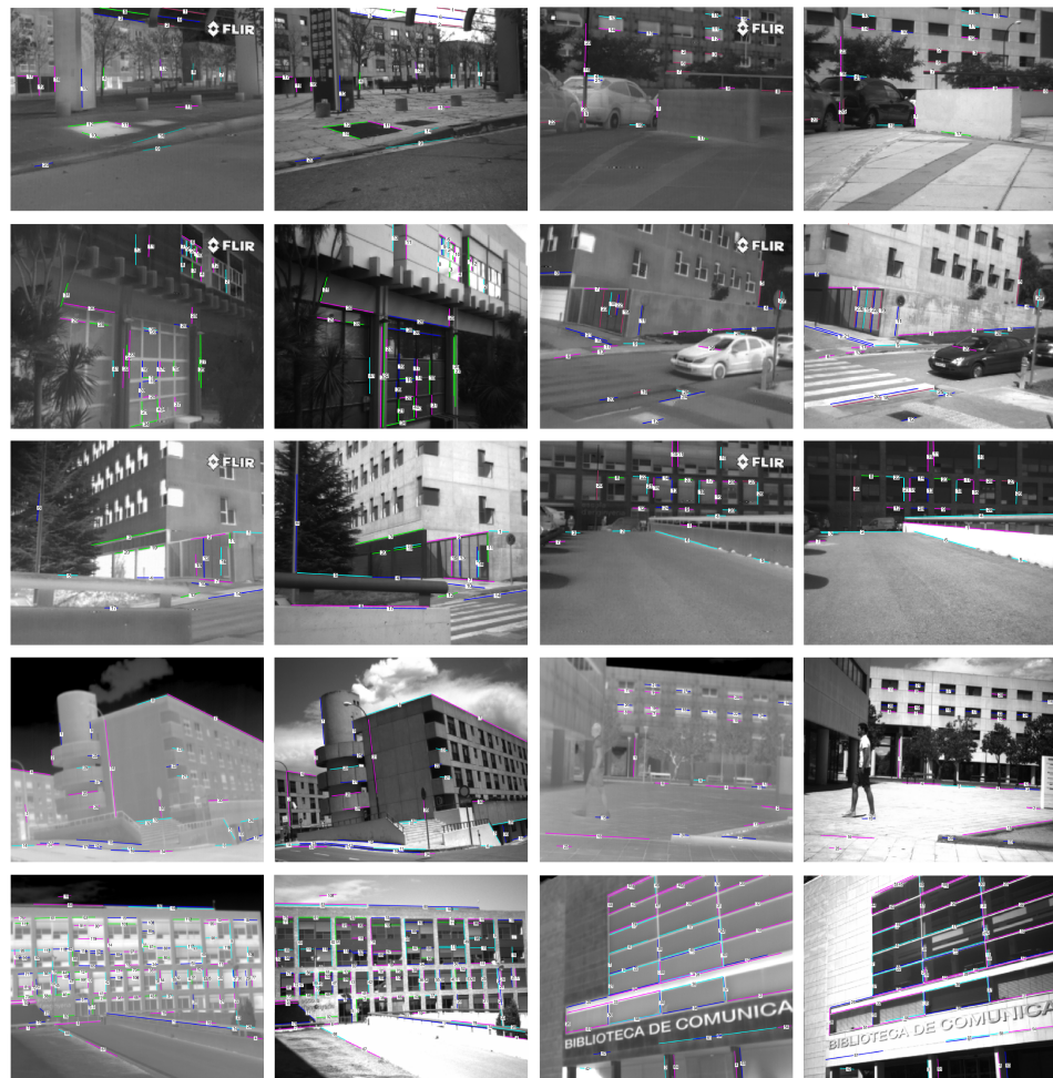
Figure 9. Demonstration of matching results of the PC-MLH (different colours mean that the matched lines are detected from different local homography layers). The images in the 1st and 3rd columns belong to LWIR images, and those in the 2nd and 4th columns are VS ones.
