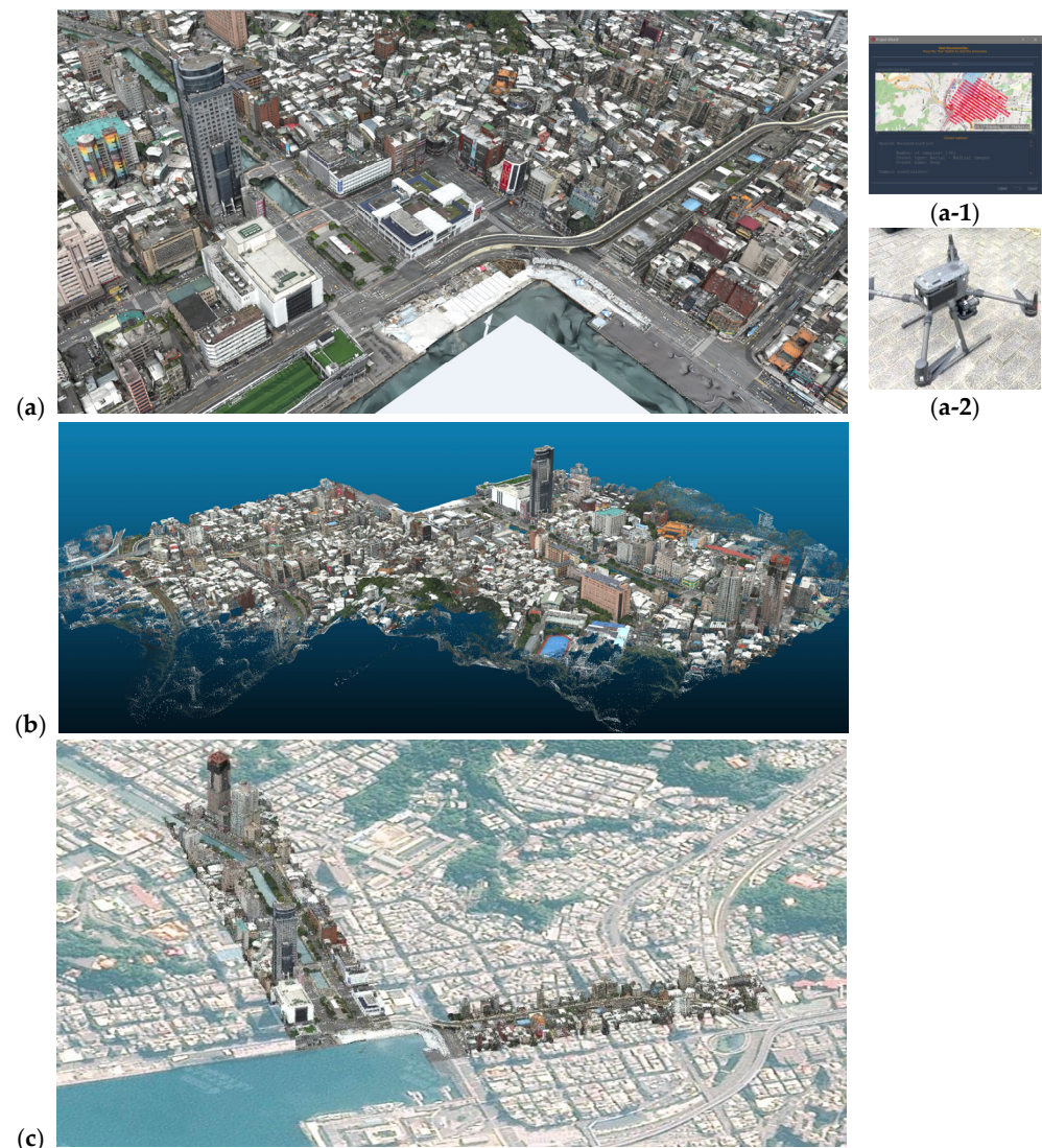
Figure 4. (a) 3D photogrammetric mesh model made by UAV images and Zephyr ® ; (a-1) UAV plan; (a-2) DJI Zenmuse P1 ® ; (b) 3D point model of inner harbor area rendered in CloudCompare ® ; (c) QGIS ® 3D layer with georeferenced 3D point models of Asahikawa River and Tianliao River.
