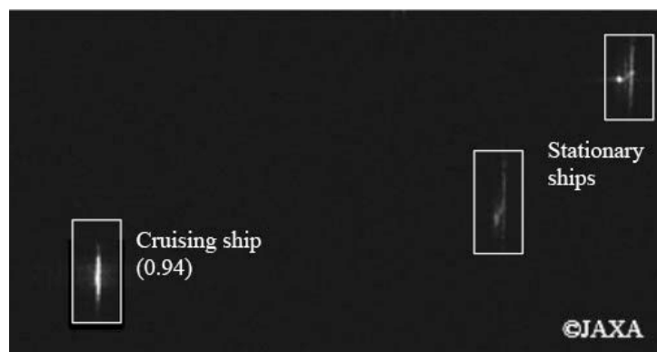
Figure 4. Example of detecting cruising ships and avoiding stationary ships. The left bottom image within the white bounding box is a cruising ship successfully detected with a high confidence score of 0.94. The right two images of ships are defined as stationary.
