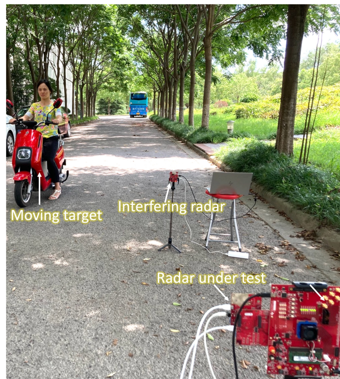
Figure 9. Real radar field experiments.
