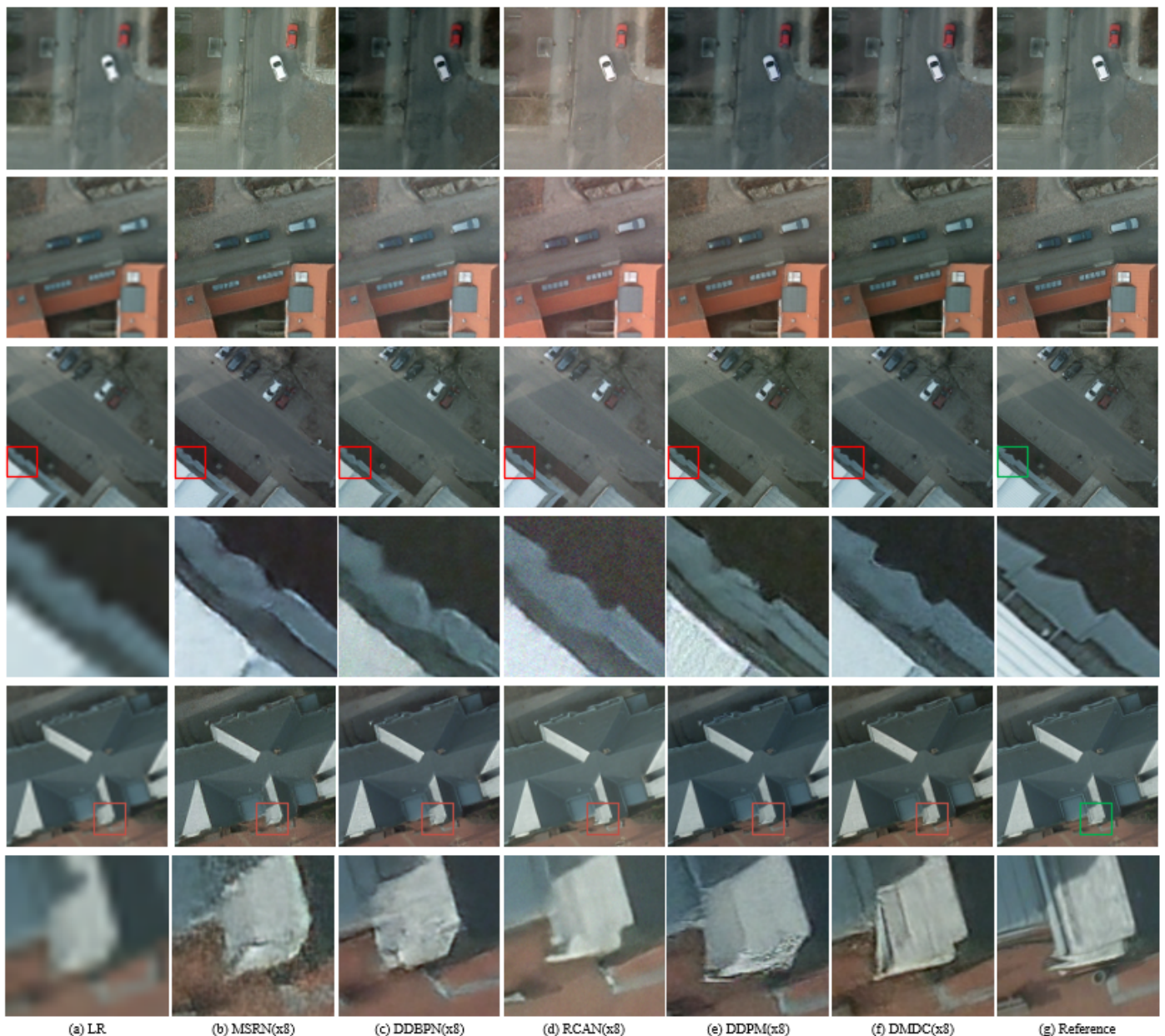
Figure 8. ISPRS-Potsdam dataset \times 8 magnification SR qualitative results. From left to right: (a) LR image, (b) MSRN [58], (c) DDBPN [59], (d) RCAN [60], (e) DDPM [18], (f) DMDC (ours), and (g) Reference. For detailed comparison, the red rectangle is cropped and its enlarged version is placed in the lower row. Compared to MSRN [58] and RCAN [60], DMDC produces more detailed and contrasting images, avoiding the artifacts encountered by DDBPN [59] and DDPM [18] (e.g., within the red boxes in row 2 and row 3, the detail recovery at the edge of the house), and maintain consistency with the ground-truth. Zoom-in for better details.
