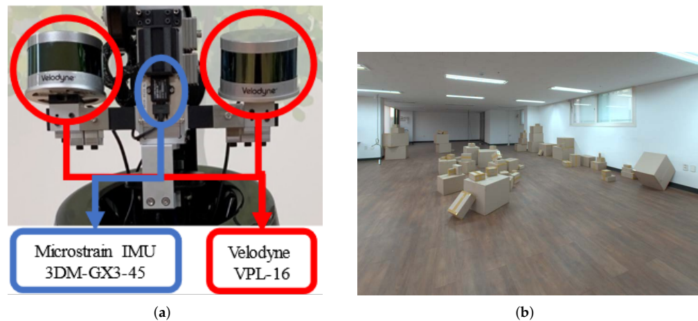
Figure 8. Real data acquisition setting. (a) Sensor system configuration. Sensor system used to acquire point clouds is consisting of two Velodyne VLP-16 channels and Microstrain 3DX-GX3-45 model. (b) Environment in which SLAM is executed to obtain real point cloud data of cuboid.
