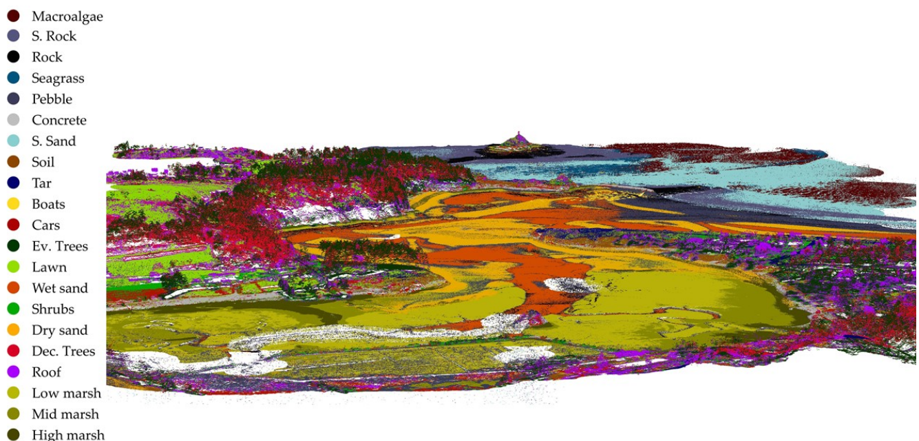
Figure 14. 3D map of the habitats obtained over the complete study area by the random forest classifier trained on green waveform features, infrared intensities, and elevations. S. = submerged, Ev. = evergreen, Dec. = deciduous.
