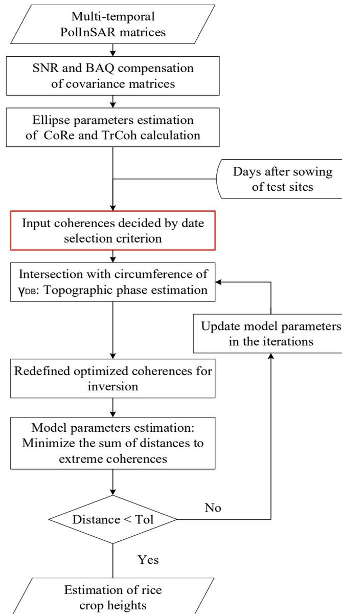
**Figure 4.** Flowchart of the time-series RVoG model based on the logistic growth equation.
