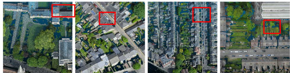
Figure 3. Part of the point cloud data (with missing data) in the SensatUrban dataset. The blue dots correspond to missing information, such as that shown in the red boxes.
