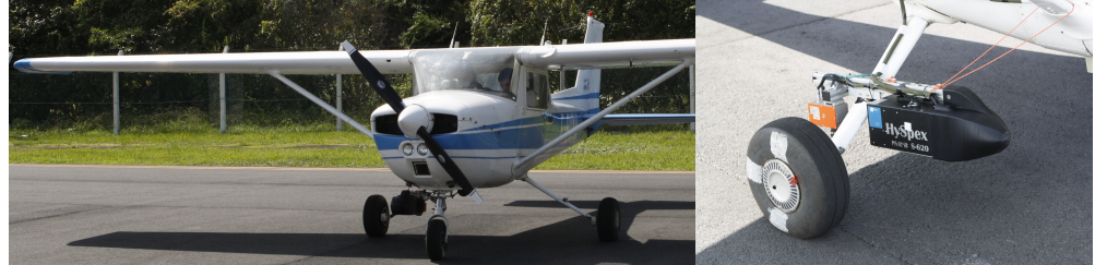
Figure 5. On the left -hand side image, the F-BUMA aircraft, and on the right side of the image, the hyperspectral imaging payload installation on aircraft landing gear.
