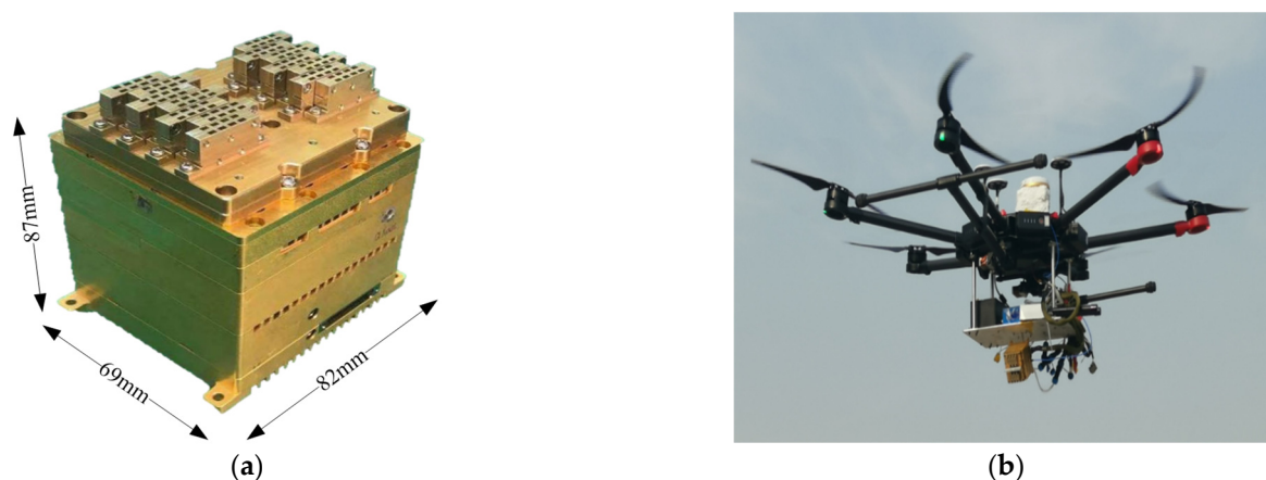
Figure 13. The W-Band APA mini-SAR and the photography on UAV. (a) The prototype of the W-Band APA mini-SAR. (b) The W-Band APA mini-SAR on the UAV platform.
