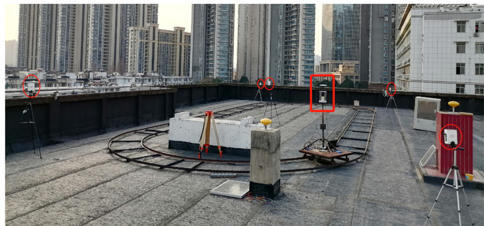
Figure 5. GNSS RTK/UWB/DBA fusion dynamic cart positioning experiment site (UWB BSs are in the red round box, and the GNSS antenna, UWB Tag, and BMP280 barometer combined device are in the red rectangular box).
