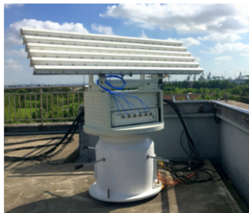
Figure 2. The ground-based MIMO radar system for LSS target detection.
