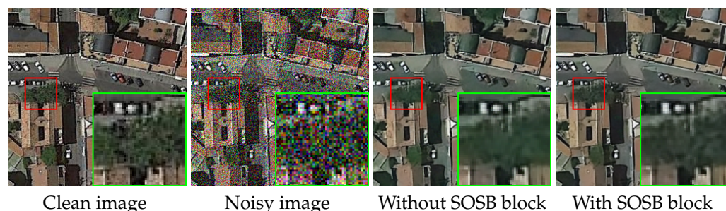
Figure 21. Enlarged detail comparisons of with/without SOSB block modules (with white Gaussian noise level \sigma^2 = 50 ).
