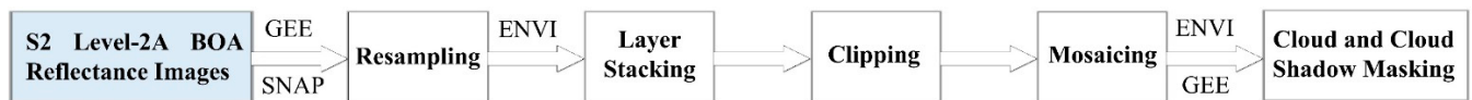
Figure 3. Preprocessing flowchart of the Sentinel-2 data, where GEE denotes Google Earth Engine ( https://earthengine.google.com (accessed on 26 April and 13 July 2022)), SNAP denotes SNAP ® software ( https://step.esa.int/main/toolboxes/snap/ (accessed on 2 and 5 November 2021)), and ENVI denotes ENVI ® software ( https://www.l3harrisgeospatial.com/Software-Technology/ENVI (accessed on 27 July 2021)).
