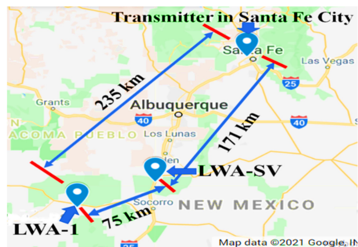
Figure 4. The distance between the transmitter and both LWA stations as well as the distance between LWA-1 and LWA-SV.
