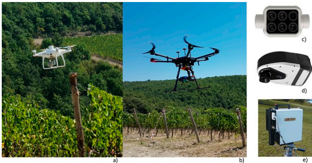
Figure 2. UAV platforms DJI P4M (a) and Matrice 600 Pro (b) used in this research to perform multispectral and hyperspectral sensing, respectively. Optical sensors used in this research: P4M multispectral camera (c), SENOP HSC-2 hyperspectral camera (d) and GER3700 spectroradiometer (e).
