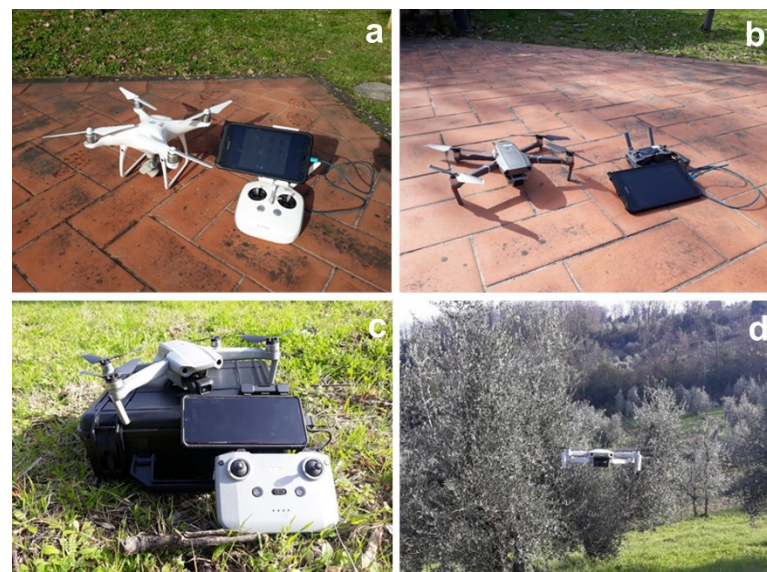
Figure 1. Used UASs: (a) Phantom 4 ADV; (b) Mavic 2 Pro; (c) Mavic Air 2; (d) Mavic Mini 2.
