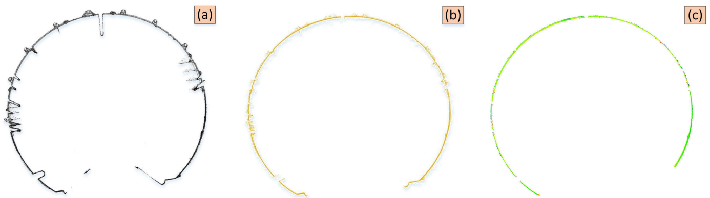
Figure 9. Point cloud filtering of tunnel section: (a) source point cloud; (b) ellipse fitting filtering; (c) model iterative filtering.
