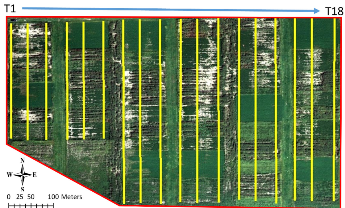
Figure 3. Geophysical data were acquired along 18 traverses, shown as yellow lines. T1 and T18 are the first and eighteenth traverses, respectively.
