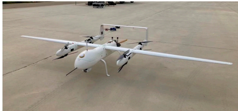
Figure 7. A VTOL industrial hybrid UAV weighs 50 kg, for carrying the entire real-time object search system.
