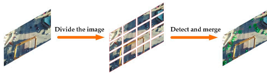
Figure 10. The aerial image is first divided into small images of equal size with overlap for detection and then merged after all of the detection is completed.
