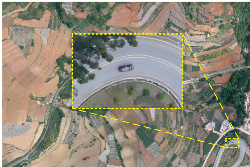
Figure 2. Small object in aerial image with a large field of view. The pixels of the vehicle in this image only account for 0.0075% of the whole image pixels. Although it is very efficient to search for objects by collecting large field view aerial images, it poses a challenge to real-time requirements.
