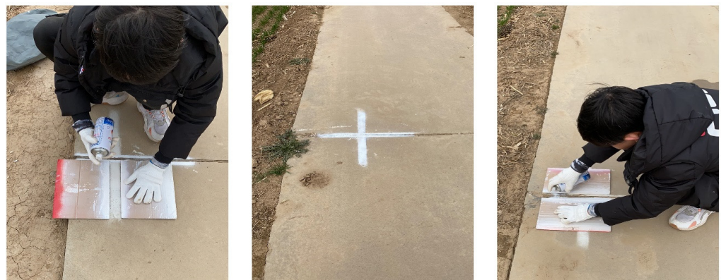
Figure A2. The detailed information of the Ground Control Point (GCP). The GCP was made using white paints, and the locations were measured using S86 system.
