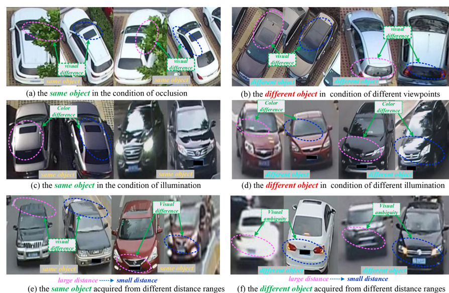
Figure 1. Illustration of parts of the challenges faced by UAV-based object Re-ID platform: (a) object appearance ambiguity by occlusions; (b) viewpoint variance resulted in dramatically different appearances of the same object; (c) illumination variance led to appearance ambiguity of the same objects; (d) illumination variances led to appearance ambiguity of the different objects; (e) resolution variances led to a visual difference of the same objects in different distances; (f) resolution variances led to the visual difference of the different objects in different distances.
