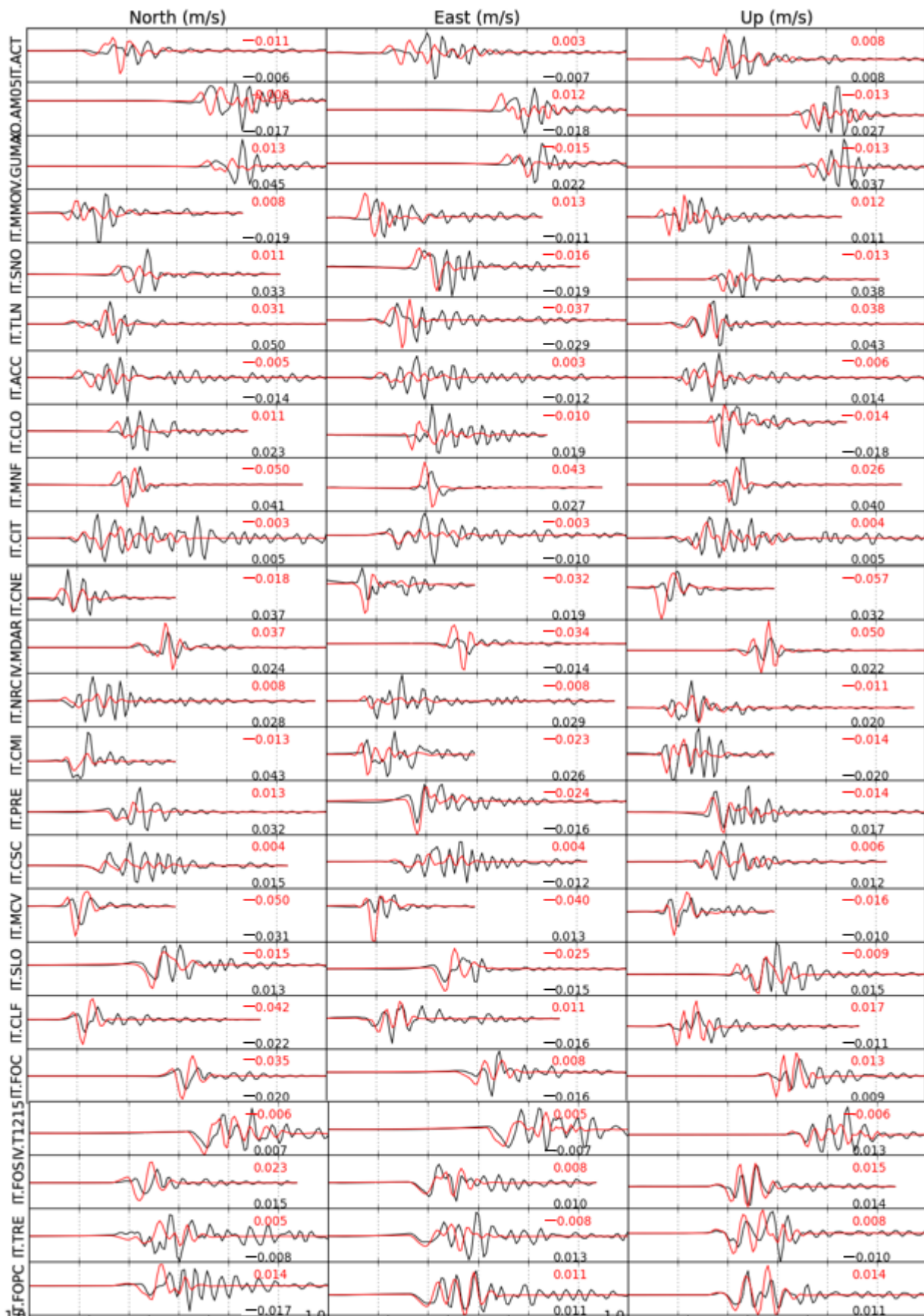
Figure A8. Comparison of strong-motion velocity records (black) and the synthetic seismograms (red) predicted by the joint slip model of the Visso earthquake.
