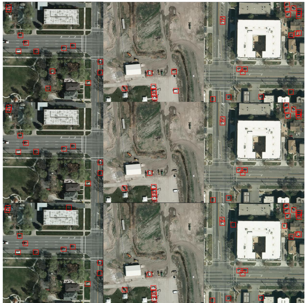
Figure 5. The detection results of the baseline model trained on the Utah city dataset. The top, middle, and bottom rows show the bounding boxes of GT, YOLOv3, and Mask R-CNN outputs, respectively.
