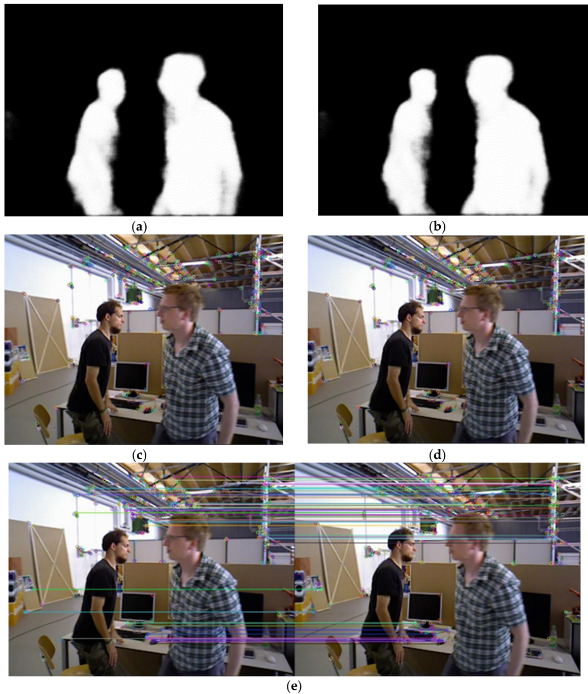
Figure 10. Results of feature extraction and matching based on proposed SLAM: (a) Figure for dynamic dot culling of first frame; (b) Figure for dynamic dot culling of second frame; (c) Feature points extracted after screening of first frame; (d) Feature points extracted after screening of second frame; (e) The ORB matching results of original Figures 1 and 2 after screening.
