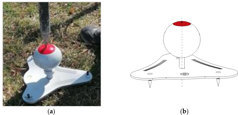
Figure 4. Author's reference sphere for TLS and UAV measurements (a) Reference sphere during measurements (b) Construction of the proprietary reference sphere.
