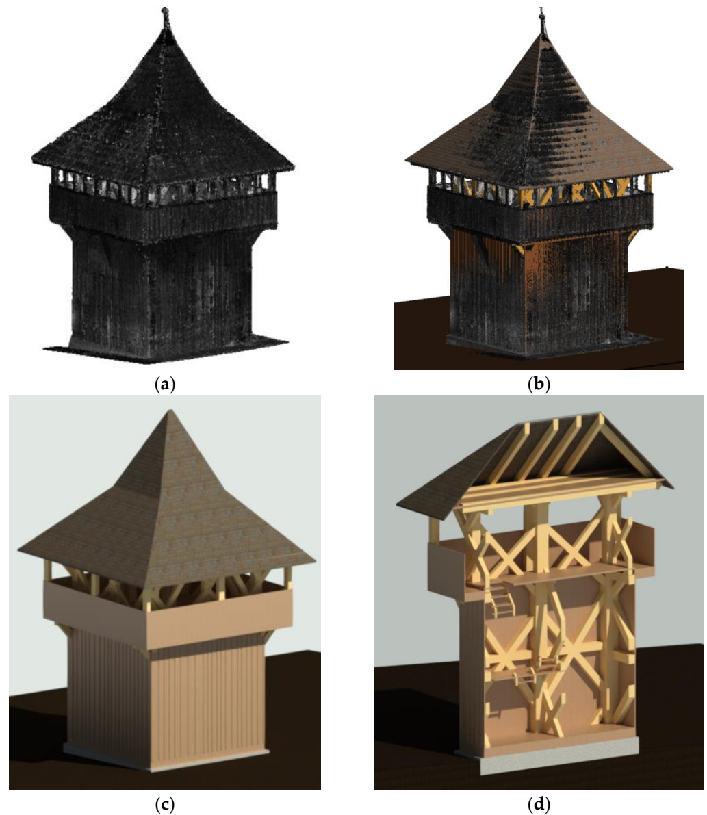
Figure 10. Work results for the belfry: (a) comprehensive point cloud with TLS-UAV integration; (b) generated model based on a point cloud; (c) visualization of the HBIM model; (d) visualization of the cross-section (interior) of the building.
