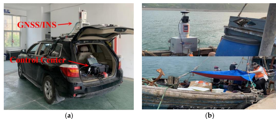
Figure 9. Experimental instrument and carriers: (a) vehicle; (b) boat.
