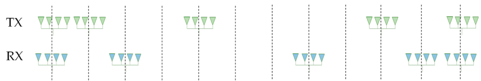
Figure 15. Non-redundant MIMO configuration. The ratios of the spacing among subarrays are 1:3:5:2 and 2:5:3:1. Each TX and RX subarray is comprised of 4 uniform arrays.
