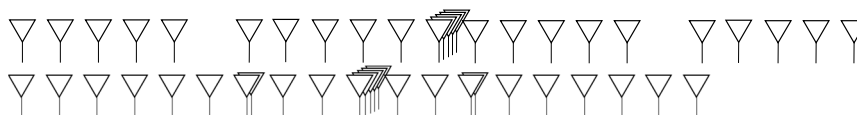
Figure 11. Non-redundant array with an interval of (1,3,5,2) can make a 23-sized VAA (up) and the MRA with an interval of (1,3,3,2) can make a 19-sized VAA (down).
