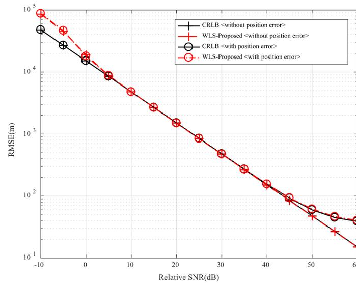
**Figure 4.** The RMSE of the target location versus the relative SNR in the presence of position errors.
