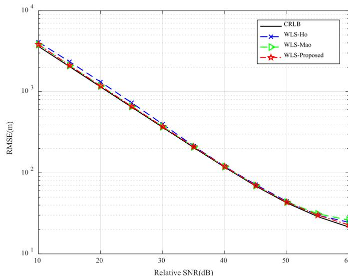
Figure 7. The RMSE of the target location versus the relative SNR under five radars.
