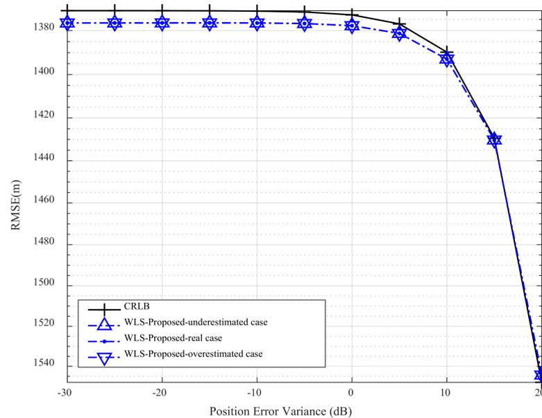
**Figure 5.** The RMSE of the target location versus the UAV position error variance under different error variance estimation cases.
