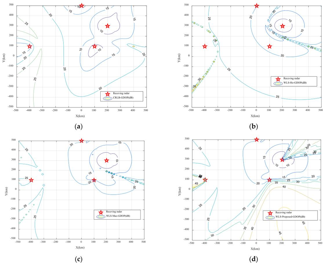
**Figure 9.** GDOP results: (a) CRLB-GDOP; (b) WLS-Ho-GDOP; (c) WLS-Mao-GDOP; (d) WLS-proposed-GDOP.
