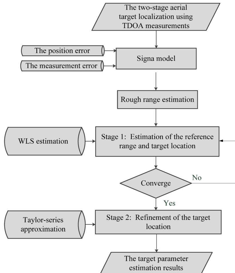
Figure 2. The flowchart of two-stage target localization method using TDOA measurements.
