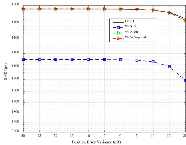
**Figure 8.** The RMSE of the target location versus the UAV position error variance under five radars.
