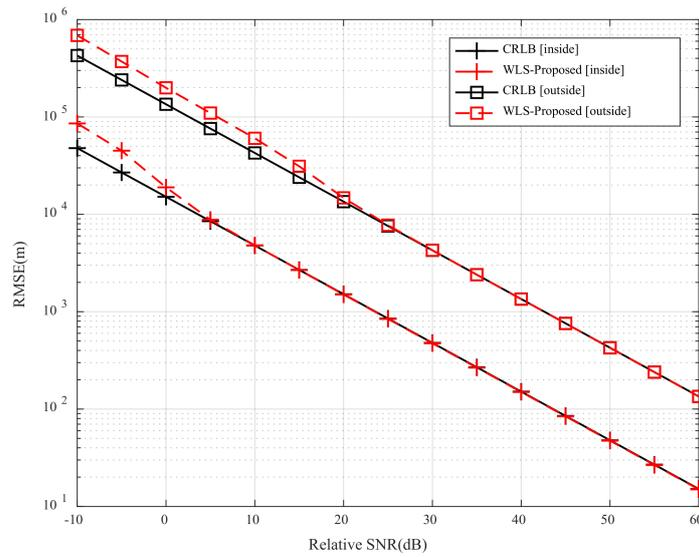
**Figure 3.** The RMSE of the target location versus relative SNR in the absence of position errors.
