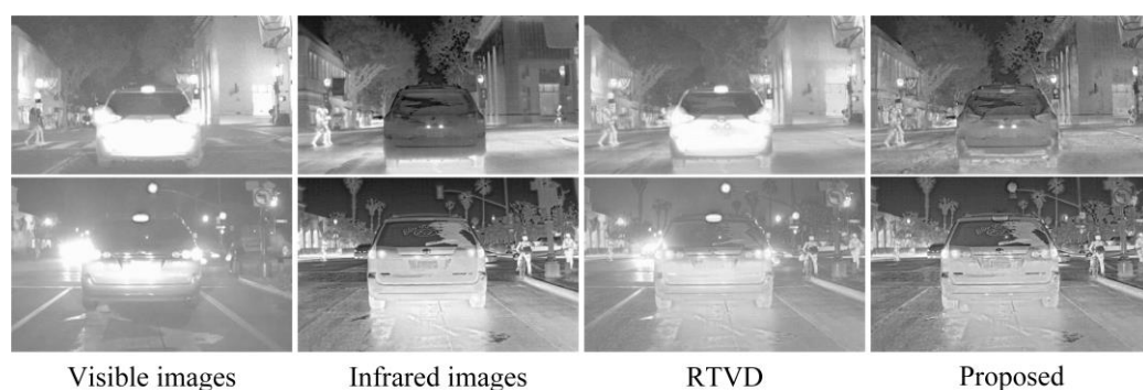
Figure 2. Results for the proposed algorithm and the comparison method, relative total variation decomposition (RTVD), on two sets of IR and visible source images.
