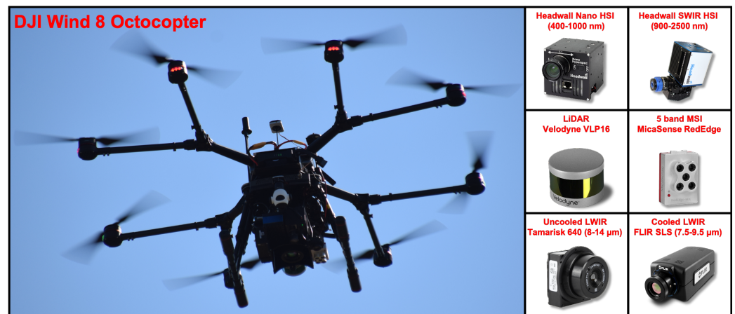
Figure 8. The MX-2 multi-modal UAS payload consisting of five different imaging sensors on-board a DJI Wind 8 Octocopter, while the SWIR HSI is on-board a DJI Matrice 600.
