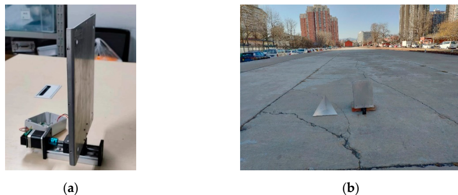
Figure 11. Photo of the vibrating calibrator and the experimental scene: (a) vibrating calibrator and (b) experimental scene.
