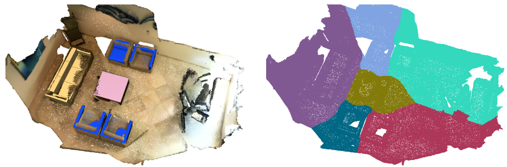
Figure 3. Sample from Scan2CAD [13] used to illustrate our method (cf. Section 4 for dataset details). (Left) Input point cloud and fitted 3D models, (right) point cloud sections which we label independently (arbitrary colors).
