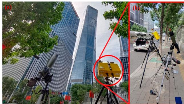
**Figure 3.** Deformation monitoring diagram of the Yunding Building. (a) Ground view of the Yunding Building from the location of the IBIS-S system; (b) View of the IBIS system on S1.
