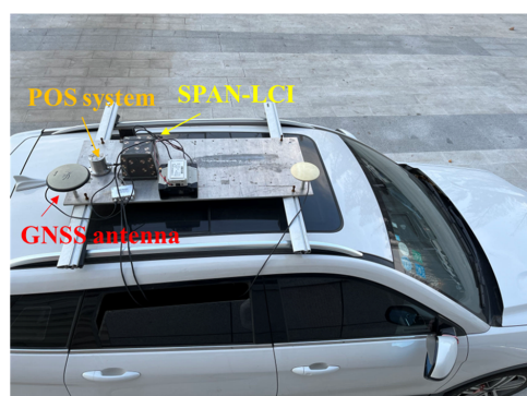
Figure 5. Experimental car and sensors.
